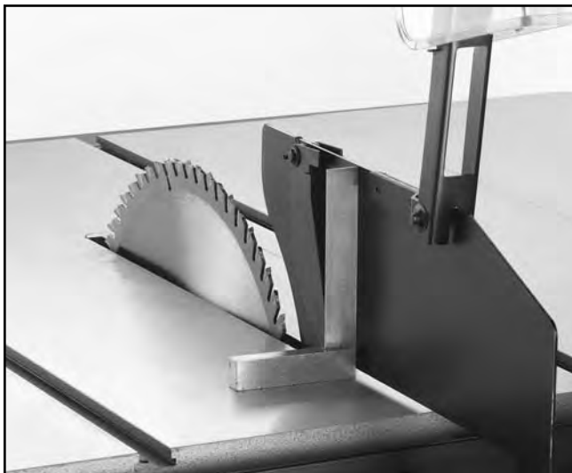
Figure 13. Guard assembly square to table.
