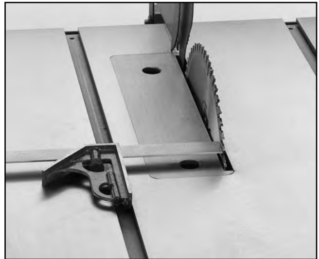
Figure 22. Adjusting blade to miter slot after rotating blade 180° and sliding square down miter slot.
