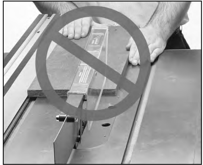
Figure 37. Do not stand directly behind wood.
