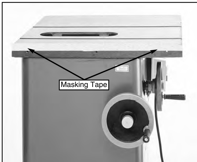
Figure 7. Using tape to shim for wing alignment.
