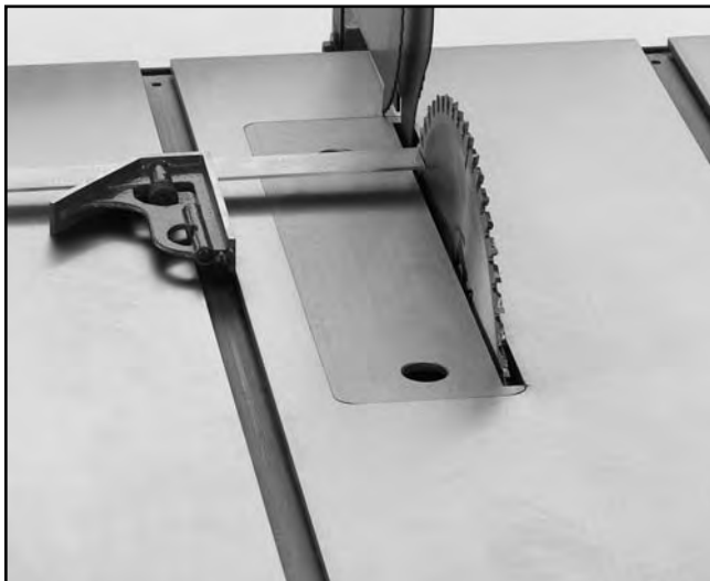
Figure 21. Adjusting blade to miter slot.
