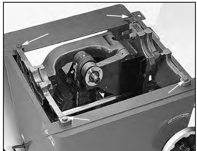
Figure 30A. Trunnion mounting bolts.
