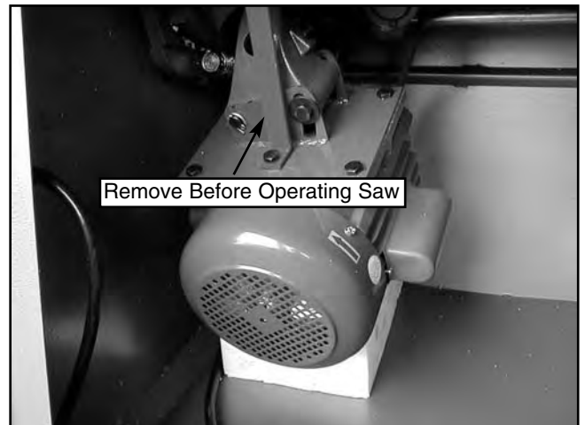
Figure 11. Remove motor bracket.
