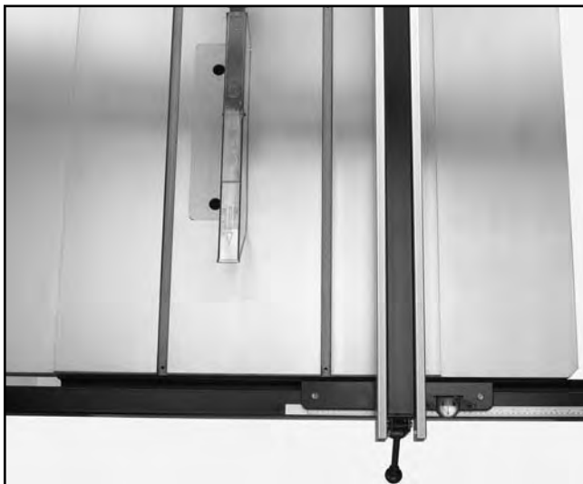
Figure 29. Aligning fence parallel to miter slot.
