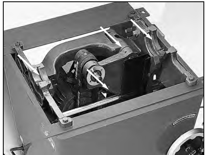
Figure 43. Lubricate these areas.
