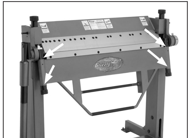
Figure 25. Location to lubricate setback threads.
