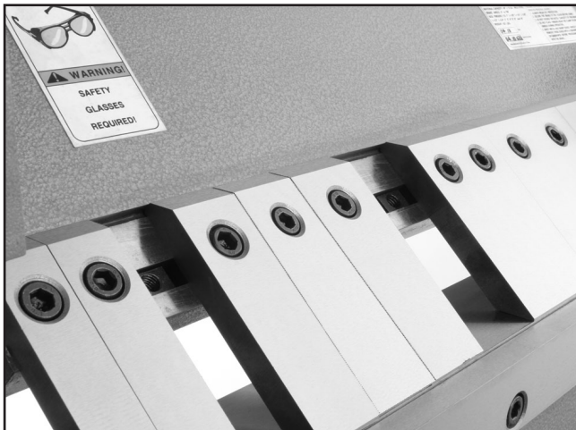
Figure 16. Fingers removed to provide space for matching fingers with box or pan widths.
