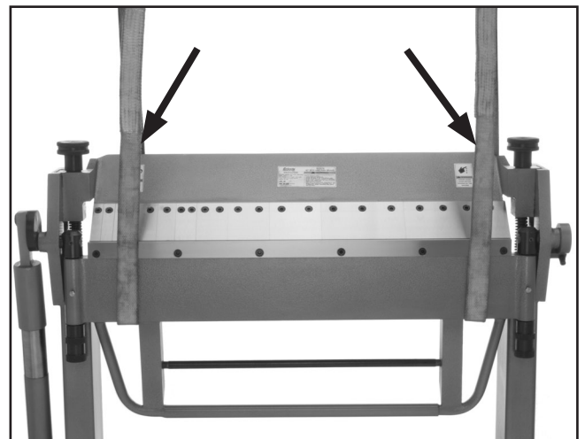
Figure 2. Typical view of a pan and box brake correctly supported evenly by two lifting straps.
