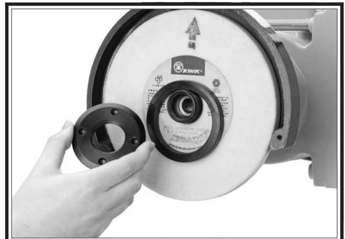
Figure 16. Exposing wheel spacer washer.
