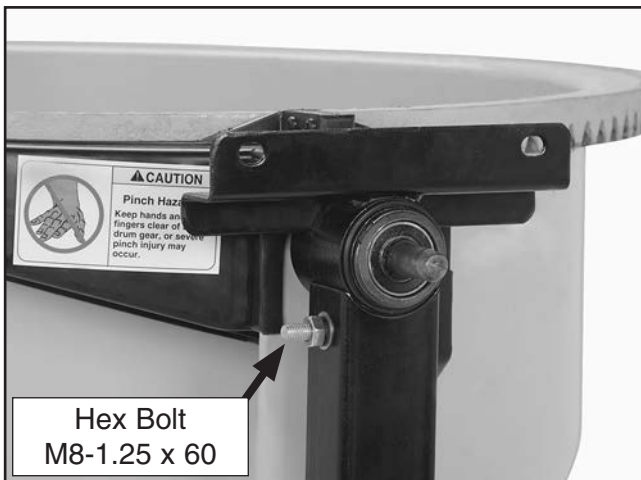
Figure 9. Bearing block installed over shaft and attached to frame.
