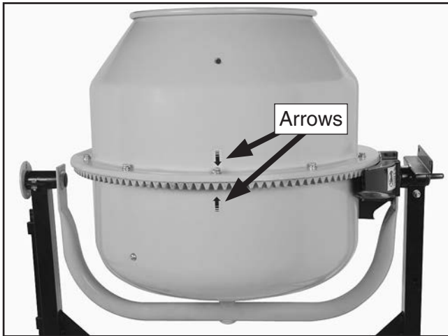
Figure 12. Upper drum attached to lower drum.
