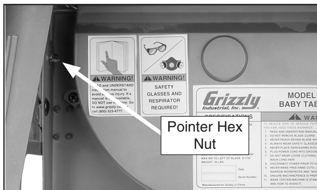
Figure 23. Pointer hex nut.
