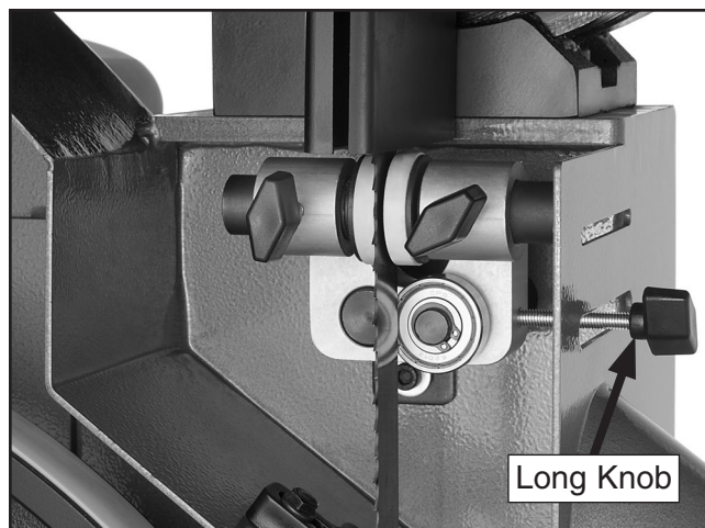
Figure 17. Long knob threaded into lower guide block.
