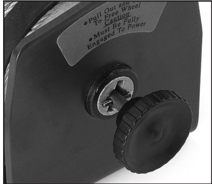
Figure 4. Clutch knob in free-spooling position.
