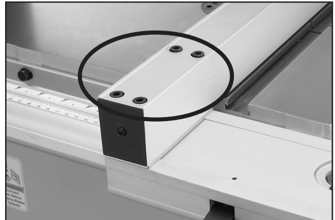
Figure 1. Four cap screws to be removed for changing fences.
