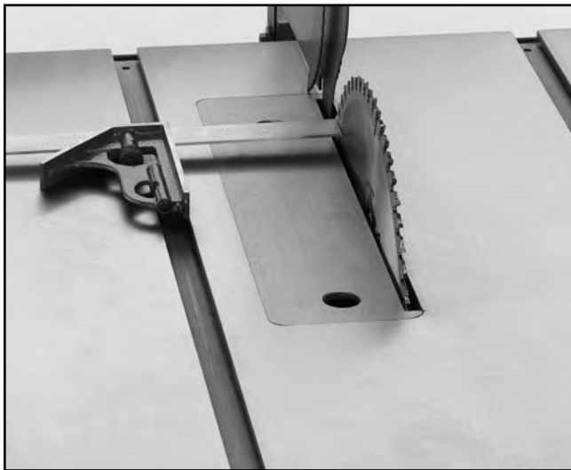
Figure 21. Adjusting blade to miter slot.
