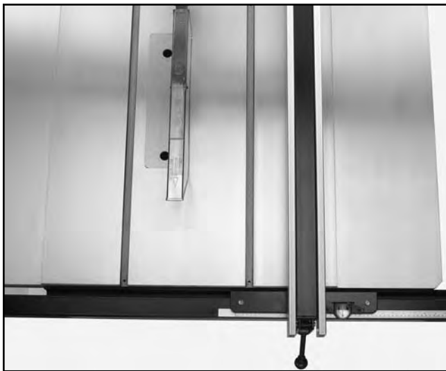
Figure 29. Aligning fence parallel to miter slot.
