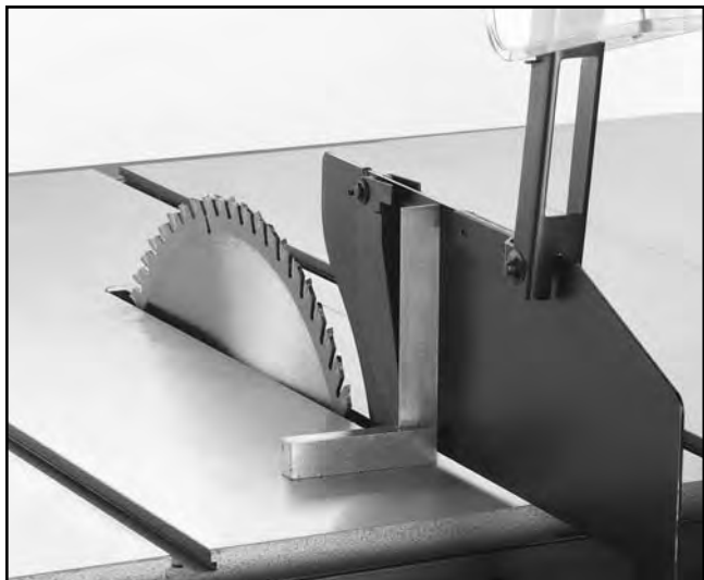
Figure 13. Guard assembly square to table.
