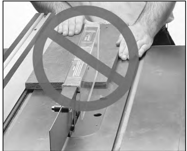
Figure 37. Do not stand directly behind wood.
