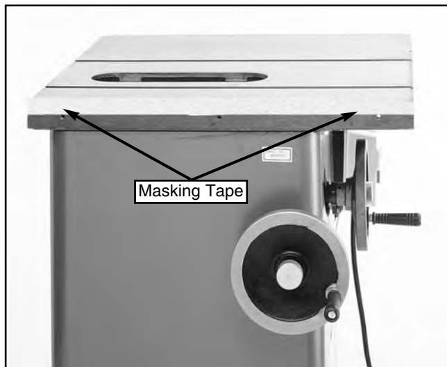
Figure 7. Using tape to shim for wing alignment.
