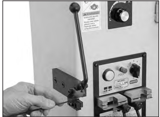
Figure 32. Using the blade shear to cut the blade.
