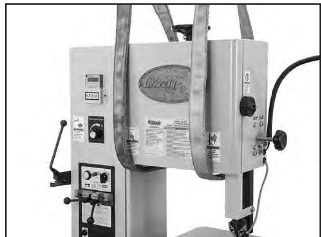
Figure 11. Lifting straps positioned on bandsaw and forklift forks.
