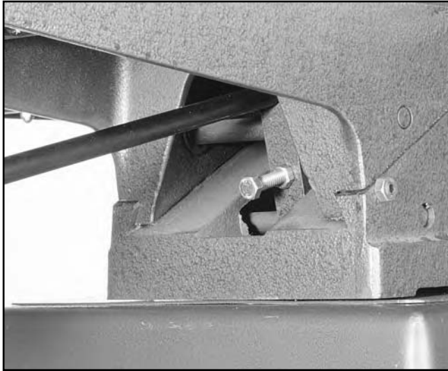
Figure 17. Table stop bolt and check nut.
