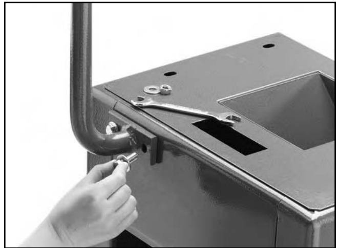
Figure 13A. Mounting pedestal switch to stand.
