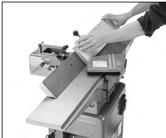
Figure 26. Fence position for bevel jointing.
