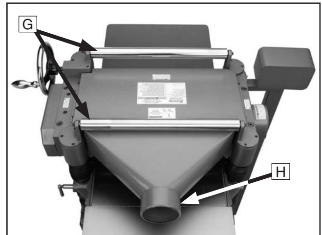
Figure 2. Return rollers and dust hood.
