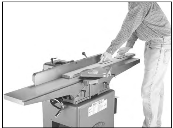
Figure 45. Surface planing the face of a workpiece.
