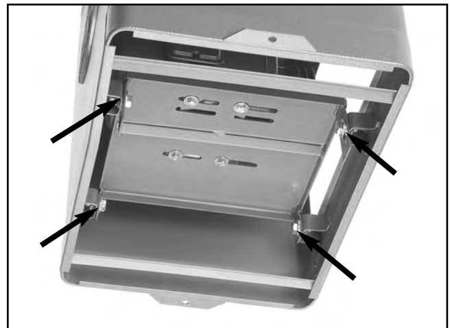
Figure 18. Motor adjustment bolts (shown underneath stand for clarity).
