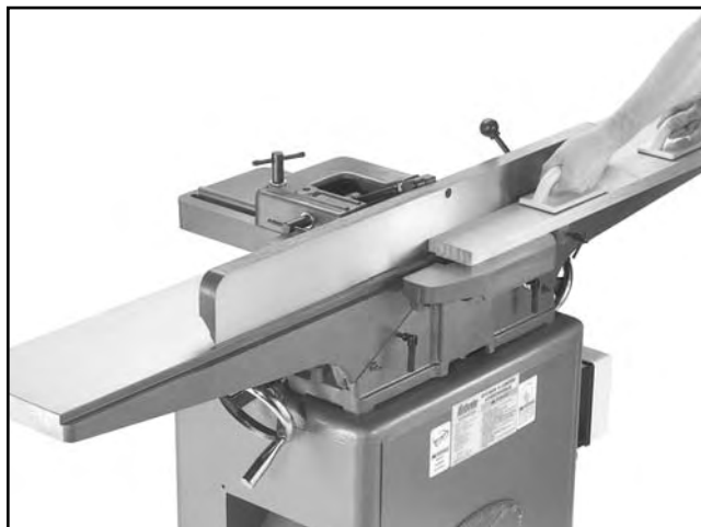
Figure 51. Rabbet cutting a workpiece.
