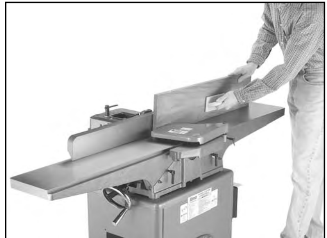
Figure 47. Edge jointing a workpiece.
