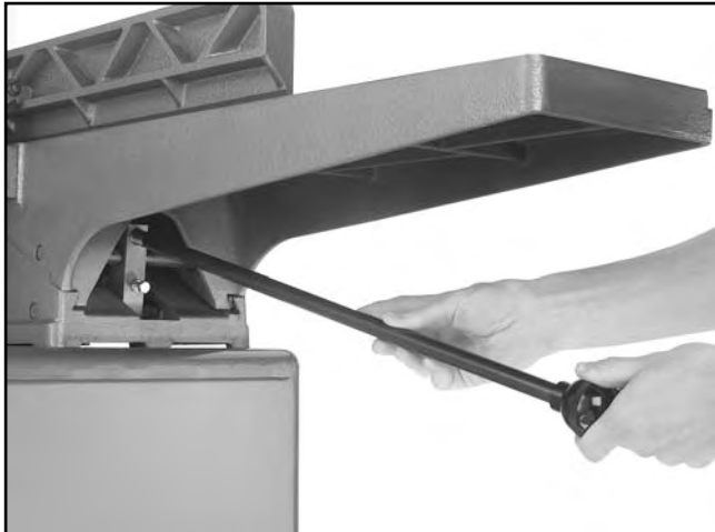
Figure 25. Installing table lever into adjustment block.
