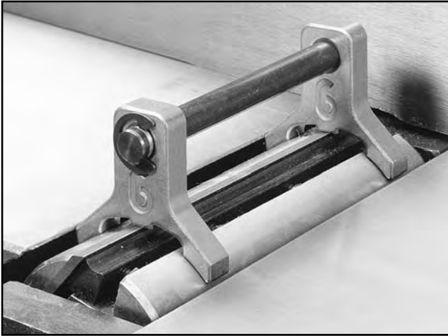
Figure 53. Jig placement on cutterhead.
