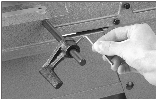
Figure 19. Installing work stop.
