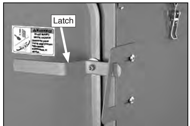
Figure 21. Properly latched door.
