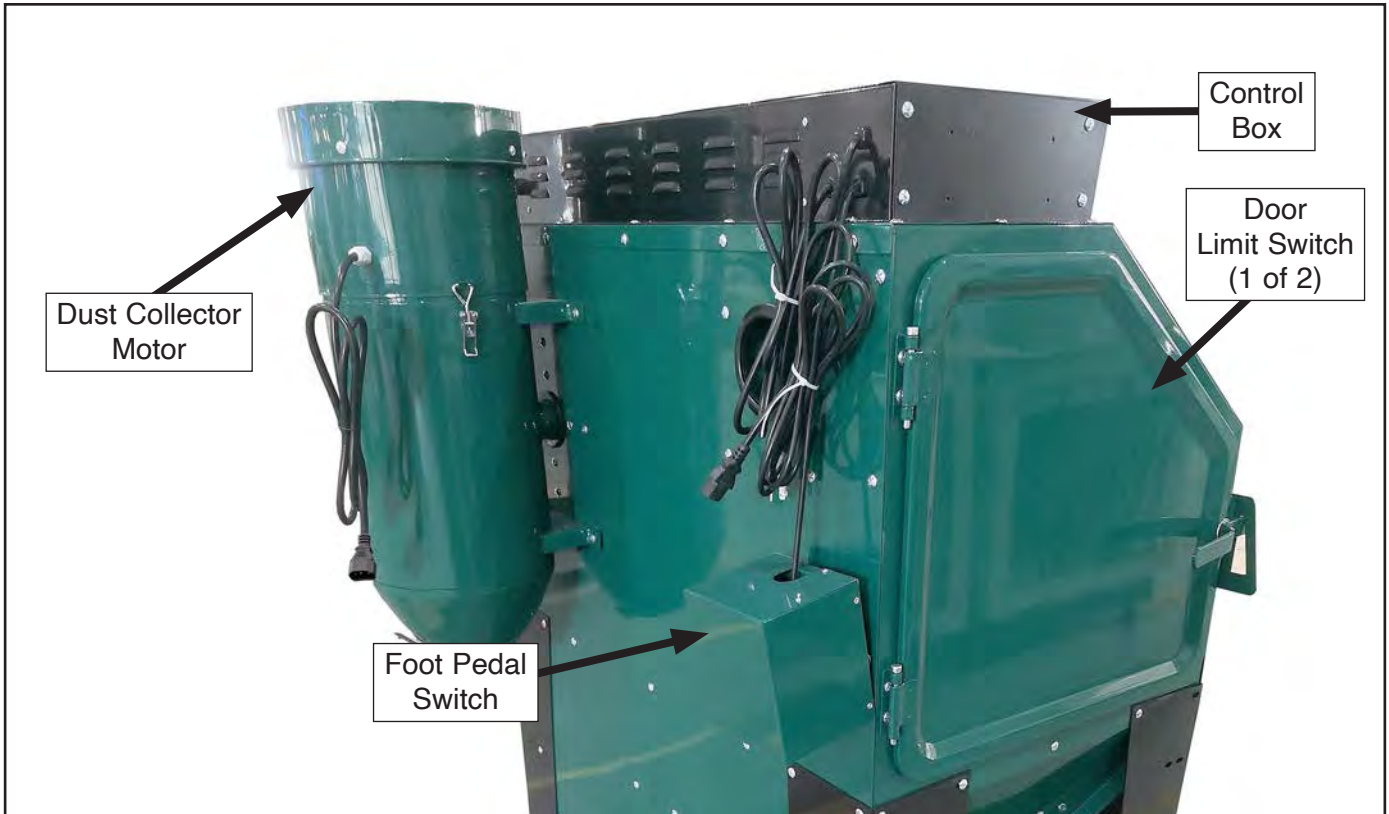
Figure 42. Locations of electrical components.
