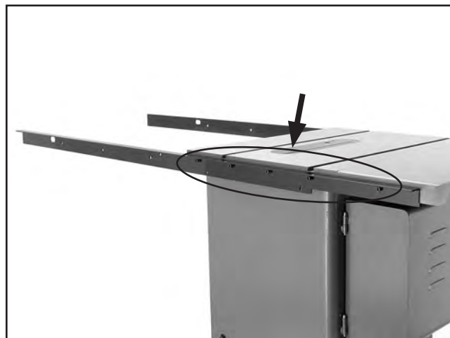
Figure 11. Rear rail installed.
