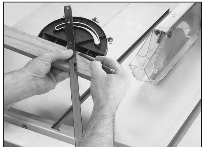
Figure 45. Example of marking miter line.
