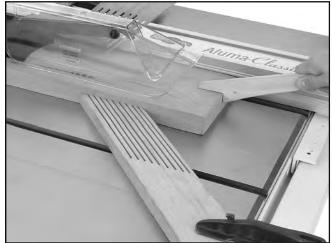
Figure 43. Typical ripping operation.
