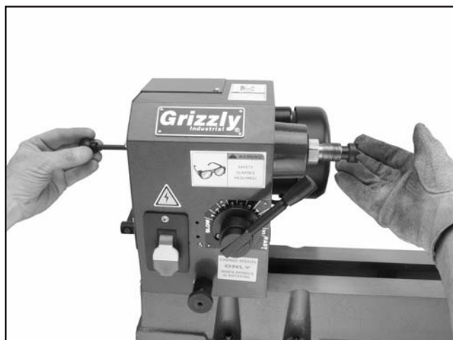
Figure 16. Removing spur center using the knock out tool.
