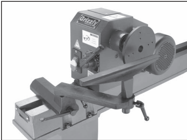
Figure 30. Headstock set at 90°.
