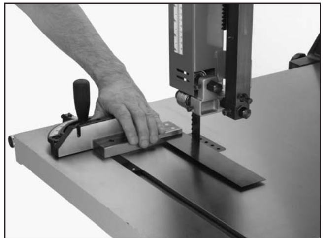
Figure 17. Squaring miter gauge to blade.
