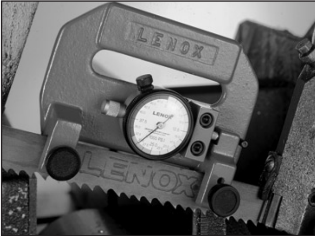
Figure 42. H5408 Blade Tensioning Gauge.
