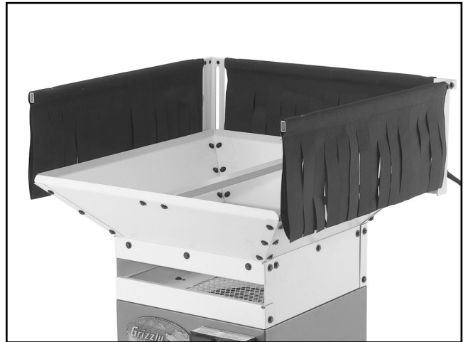
Figure 21. Curtains installed on curtain frame.
