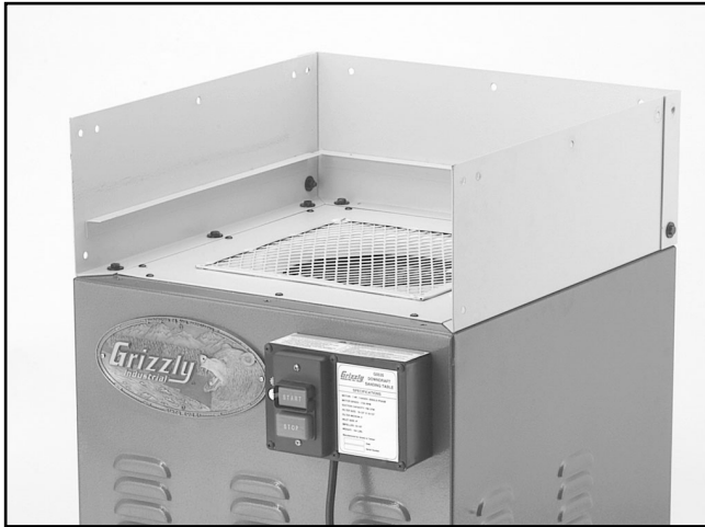
Figure 13. Side and rear filter walls installed on motor cabinet.
