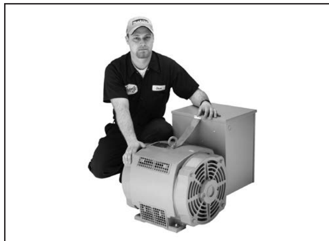
Figure 44. Typical Rotary Phase Converter
