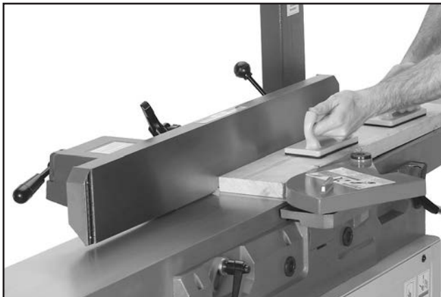
Figure 31. Example of surface planing operations.
