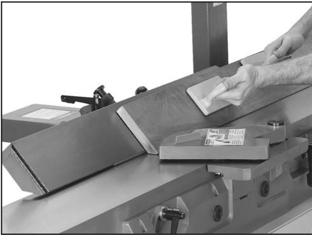
Figure 35. Fence setup for a bevel cut of 45°.
