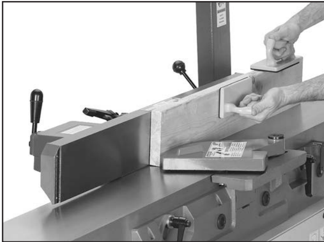
Figure 33. Example of edge jointing operation.
