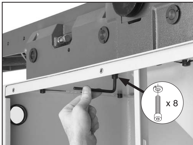
Figure 13. Securing the jointer assembly to the stand.
