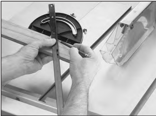
Figure 46. Marking miter line.
