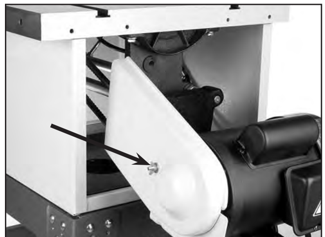
Figure 23. Installed V-belt guard cover.
